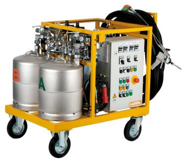
HD-2 standard version and electropneumatic refilling device
